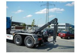
The range of the container lengths: between 3050 and 7600mm (depends on type of the hook carrier).
